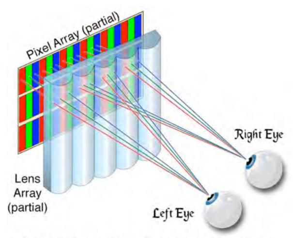
Figure 2: Lenticular Lens Array Autostereoscopic system. The microlens system steers the light path to allow each eye to see different regions of the display behind the lenses.
