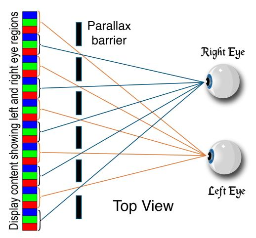
Figure 1: Parallax Barrier Autostereoscopic system (Top View). The parallax barriers are transparent and opaque strips to allow each eye to see different regions of the display behind the barrier.
